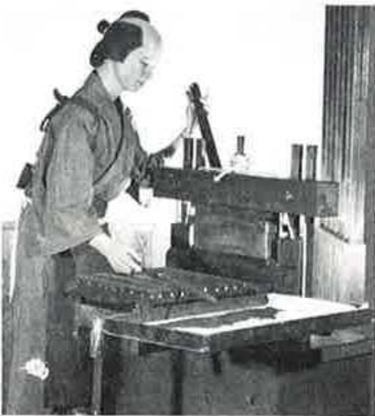
AN APOTHECARY AT WORK ON A LATE 19th CENTURY; HAND-OPERATED PILL MAKING MACHINE
